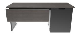
MOD2965-01 is configuration of the ModuDesk Series. It includes a modesty panel and a built in 10U rack compartment with 23" depth. The unit comes with levelers that can be swapped out with casters. The base of the rack is comes with a small lower shelf (MOD-LS), allowing air to freely flow into the unit while the cutout door handles allow for air to exit (Fans are optional if required).
